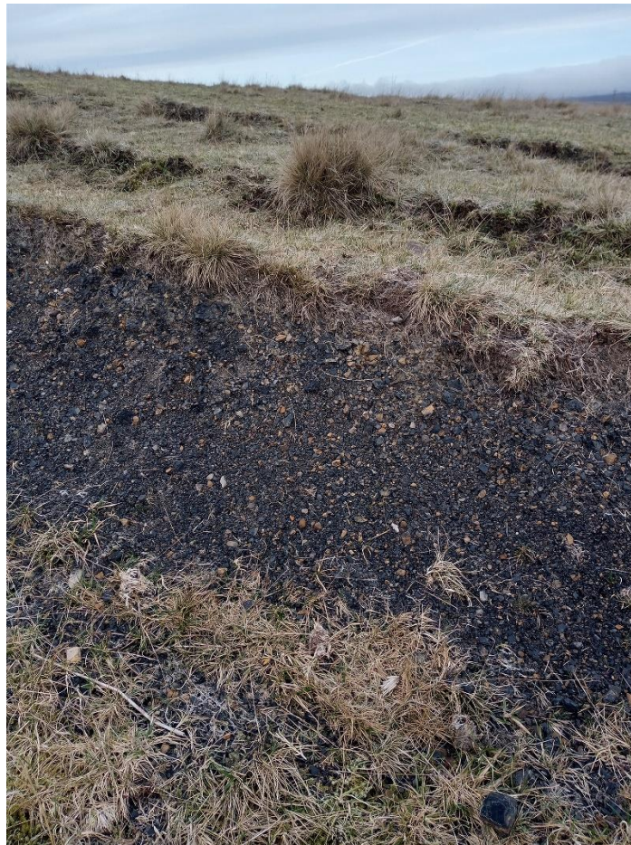
Photograph 2: Exposed soil profile due to localised erosion in Area 6. A thin topsoil layer (<10 cm) overlies a layer of opencast spoil.
