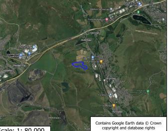
This figure shows the geographical extent of potential glint events out to 5km. For a glint event to occur on the ground the receptor must be in both the ZTV and the ground based glint zone. The ZTV is based on 2.5 m high panels, a receptor height of 1.8 m and OS Terrain 50 topographic data with  $50\ m$  resolution grid. The use of a Digital Surface Model would further reduce the extent of the ZTV.
